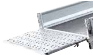
Full Ramp Door and Props
