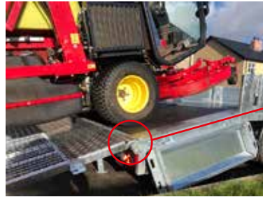
'Silent sides': Spring loaded flip latches on all drop sides prevent undue movement and noise
